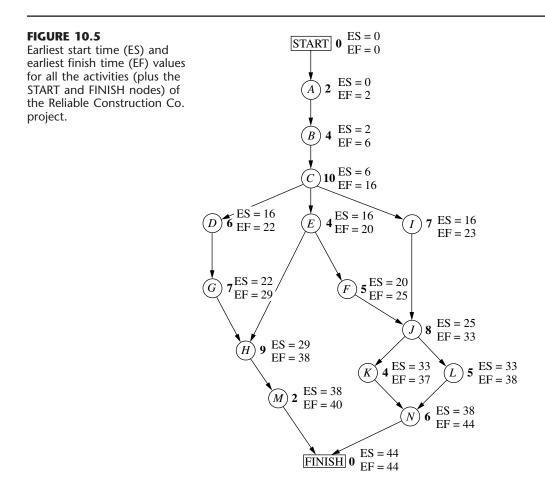
Note that Fig. 10.5 also includes ES and EF values for the START and FINISH nodes. The reason is that these nodes are conventionally treated as *dummy activities* that require no time. For the START node, ES=0=EF automatically. For the FINISH node, the earliest start time rule is used to calculate ES in the usual way, as illustrated below.
