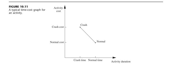
these two points. (For example, this assumption says that *half* of a full crash will give a point on this line segment that is midway between the normal and crash points.) This simplifying approximation reduces the necessary data gathering to estimating the time and cost for just two situations: *normal conditions* (to obtain the normal point) and a *full crash* (to obtain the crash point).
