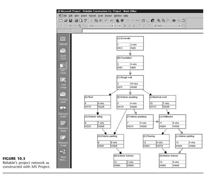
after placing the activity boxes in the same locations as the corresponding nodes in Fig. 10.1 (except no boxes are included now for the start and finish of the project). Note that each box provides considerable information about the activity. After giving its name, the second row shows the activity number and duration. The last row then gives the scheduled start and finish times.
